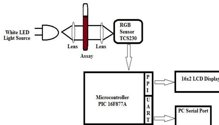
Fig.2. Block Diagram of CMOS RGB Colour Sensor TCS230 Based pH measurement system using PIC µcontroller 16F877A.
