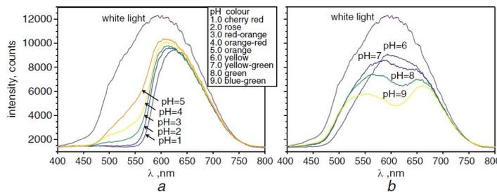
**Fig.6. Output response of liquid sample for different pH values.**
