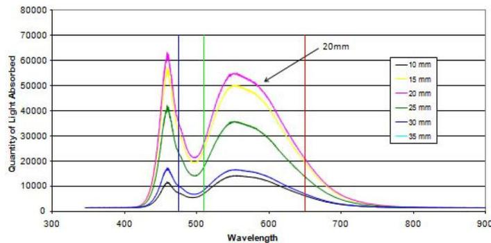
Fig.1. Light absorbed from TCS230 across the white LED light spectrum when the sensor is positioned at 6 different heights
