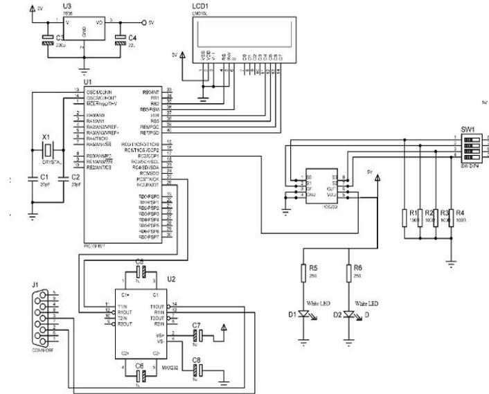
**Fig.3. Schematics of Programmable CMOS RGB Colour Sensor TCS230 Based pH measurement system using PIC  $\mu$ controller 16F877A.**
