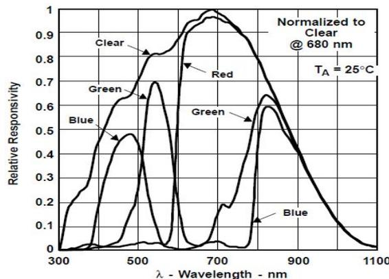
Fig.5. Photodiode Spectral Responsivity of TCS230 Sensor
